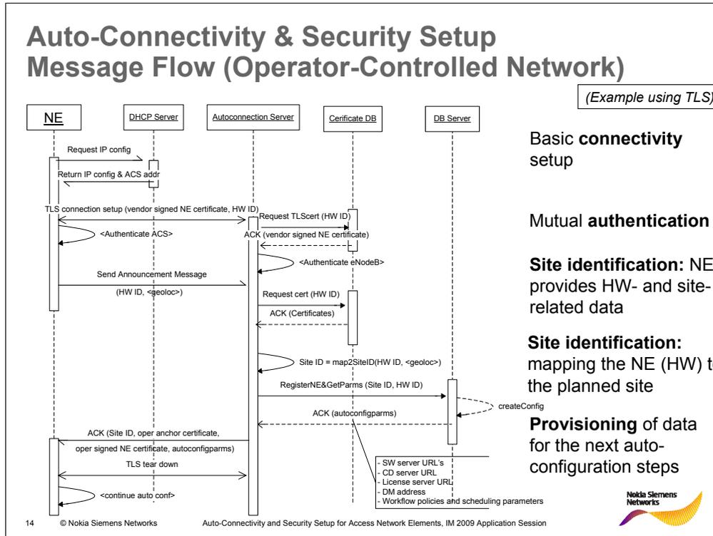
This simplified message flow illustrates the steps of the authentication and security setup, more specifically for the case with automated site identification.
